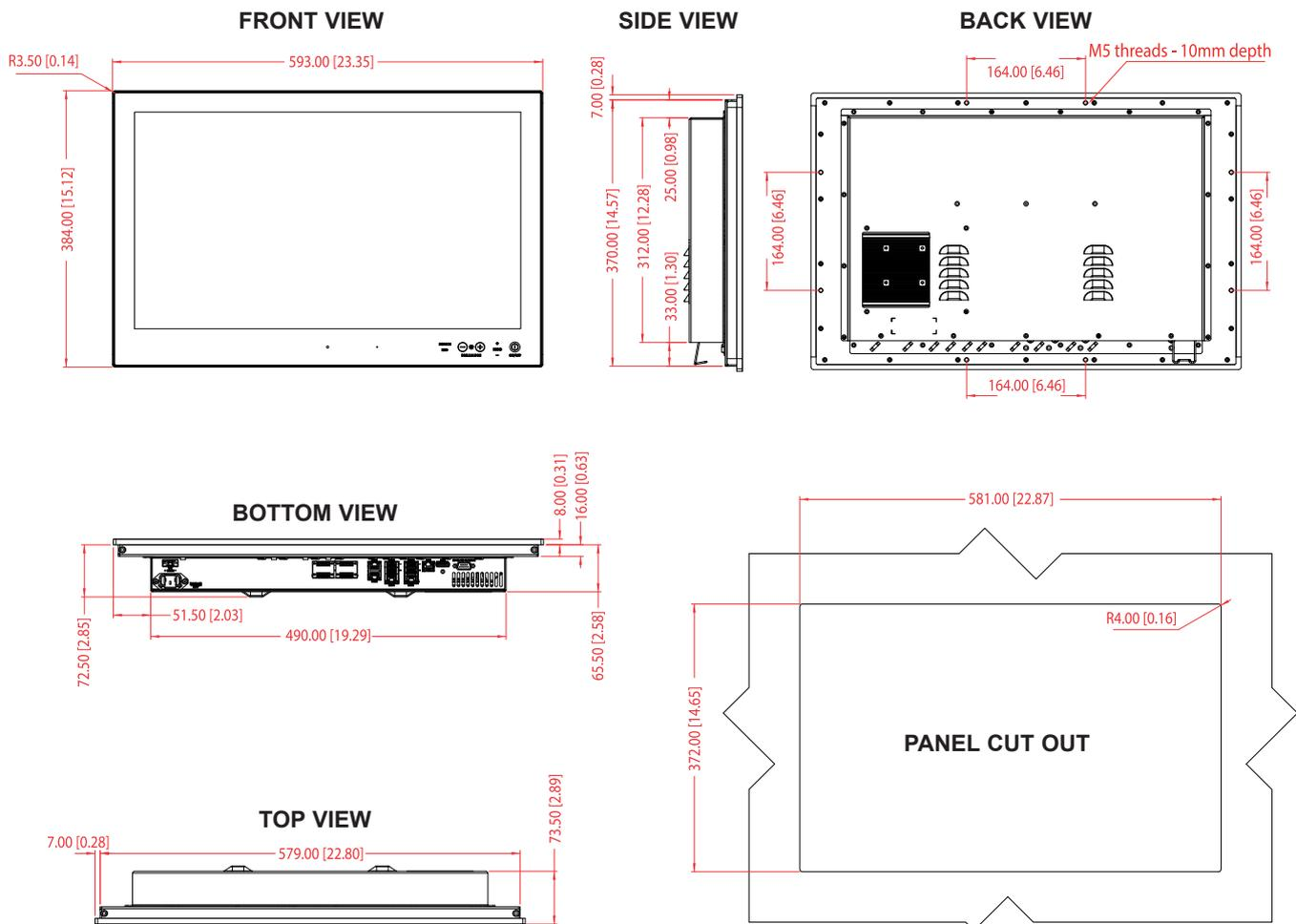
Dimensions might be shown with or without decimals and indicated as mm [inches]. Tolerance on drawings is +/- 1mm. For accurate measurements, check relevant DWG file.
